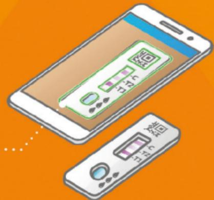
You have **2 minutes** for evaluation. Align the stencil on the display with the test cassette — hold your smartphone parallel to the test cassette. **Attention:** Make sure that the lighting is even. Avoid shadows and direct sunlight. If the time is exceeded, the result becomes **invalid**. The measurement must be repeated with a new test kit.
